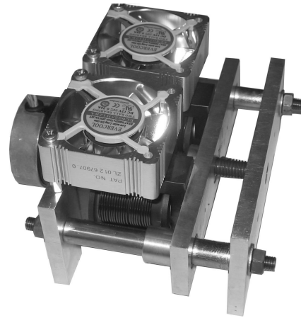
Рис. 5. Adjustable inductance with a changeable clearance in the magnetic core.
