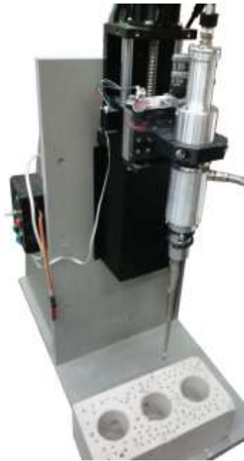
Setup for ultrasonic drilling at room temperatures
