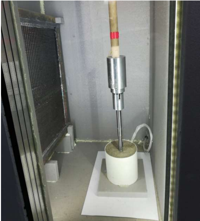
Photos of the ultrasonic drilling process at different points in time at temperature -80^{\circ}\text{C}
