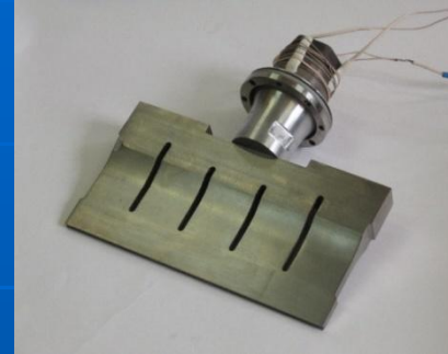
б) - two-half-wave vibratory system for seams of 220 mm;
