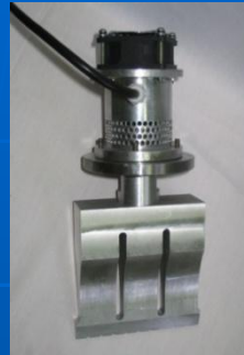
b) two-half-wave vibratory system for seams of 150 mm;
