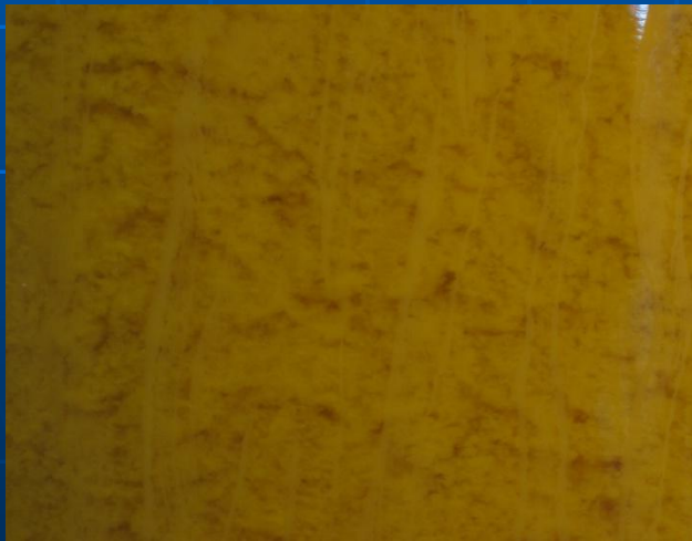
Forming of impurity shards if wine-material at settling after ultrasonic processing
