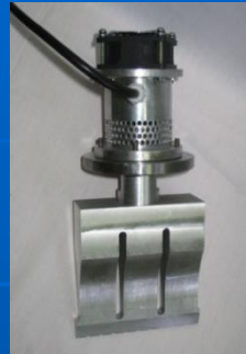
b) two-half-wave UVS for seams of 150 mm;
