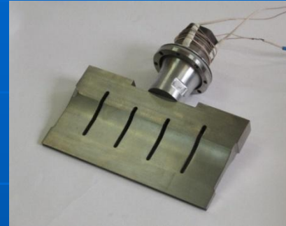
c) two-half-wave UVS for seams of 220 mm;
