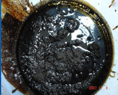
Petroleum sludge before ultrasonic processing
