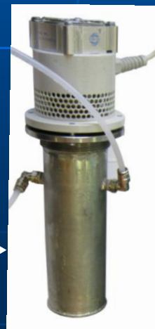
Upgraded ultrasonic radiator with a sound-conducting volume
