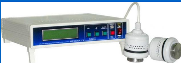
Ultrasonic laboratory device «Negnost» for processing of liquids (frequency – 44 kHz, intensity up to 4 \cdot 10^4 W/m 2 )
