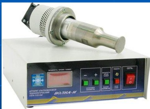
Ultrasonic industrial device “Volna-M” for processing of liquids (frequency – 22 kHz, intensity up to 20 \cdot 10^4 W/m 2 )
