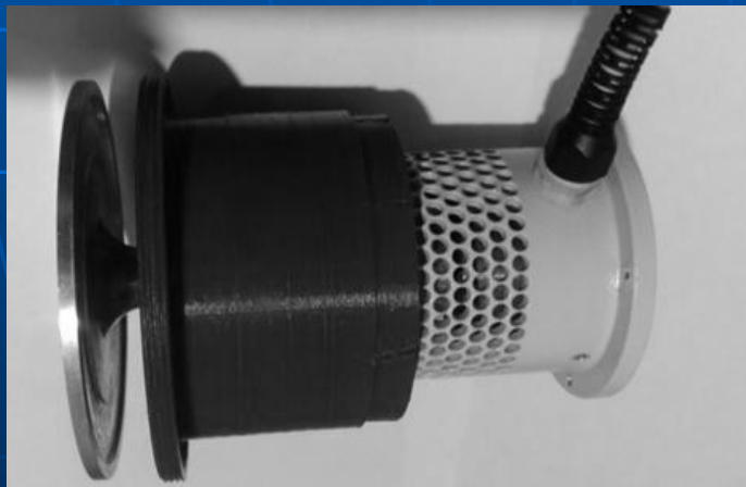
Photo of the ultrasonic vibratory system: 1 – disk radiator; 2 – piezoelectric transducer; 3 – case; 4 – flange; 5 – fan
