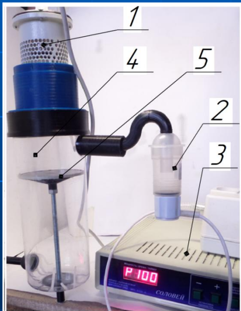
1 – ultrasonic disk radiator; 2 – aerosol generator; 3 – ultrasonic generator to supply disk radiator; 4 – coagulation chamber; 5 – reflector Stand for study of ultrasonic coagulation in standing wave mode
