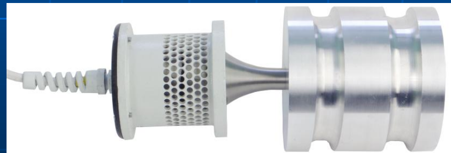
Photo of the ultrasonic vibratory system: 1 – ultrasonic radiator; 2 – concentrator of piezoelectric transducer; 3 – piezoceramic elements; 4 – reflective overlay; 5 – case; 6 – flange; 7 – pin
