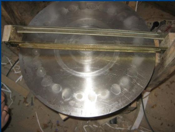
Appearance of the ultrasonic disk radiator
