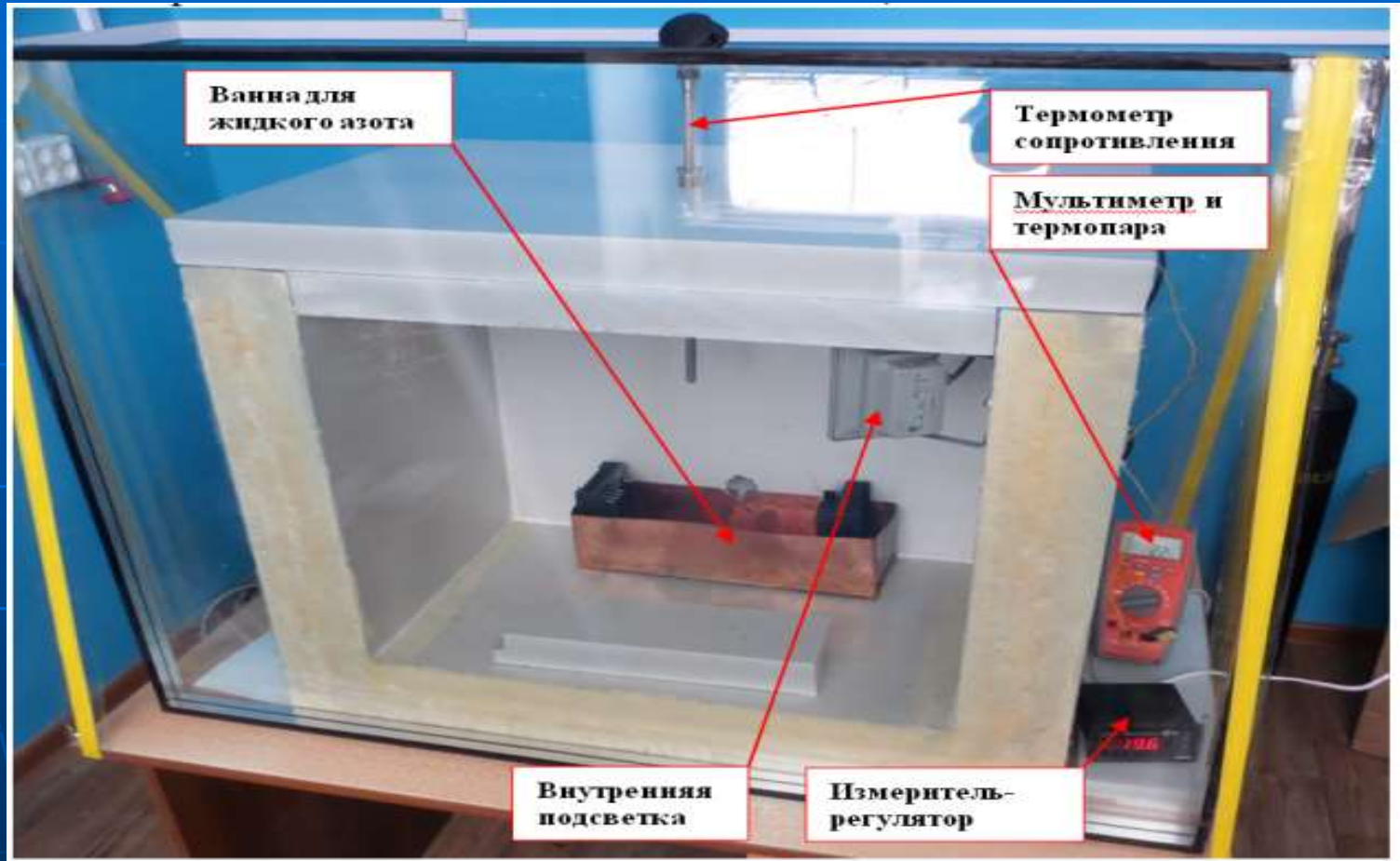
Stand for experimental studies at low temperature provided by liquid nitrogen
