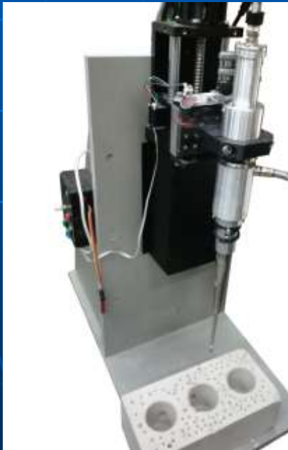
Setup for ultrasonic drilling at room temperatures
