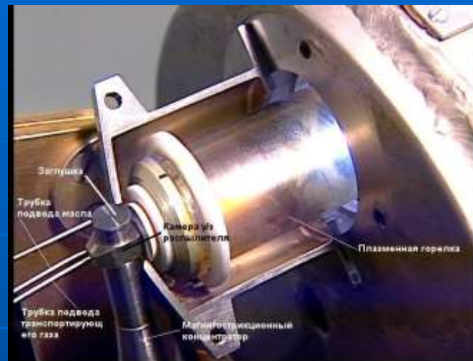
Ultrasonic atomizer mounted in a plasma burner
