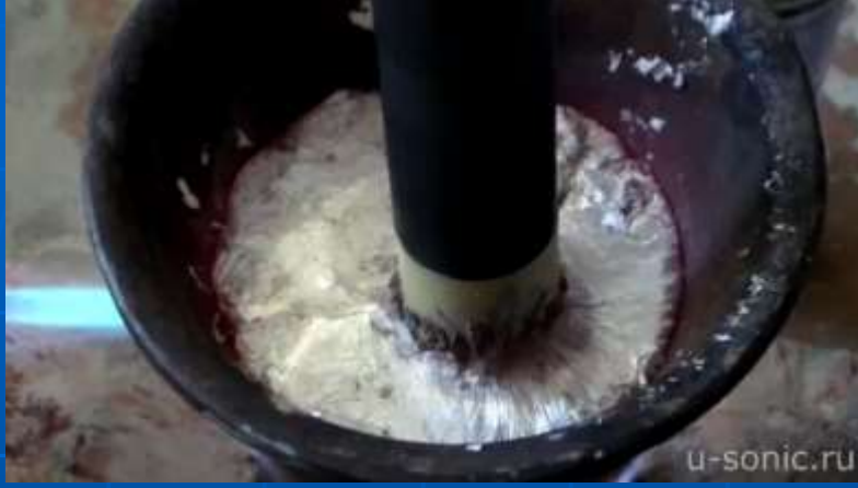
Crystallization of Al-4 % Cu without ultrasonic treatment
