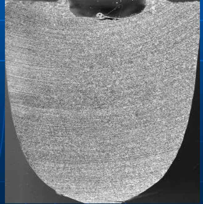
Crystallization of Al-4 % Cu with ultrasonic treatment
