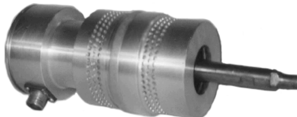
Photo 2 – Rotation system with gyrating transformer
