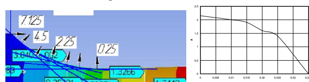
Fig. 5 – The distribution of the vibration amplitude on the radial junction of the radiating element
